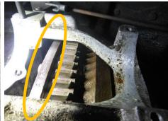
The original starter fitted to the vehicle pulls its bendix in to the ring gear from the gearbox side therefore is obviously unaffected.
