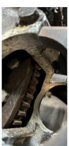
The WOSP LMS1248 engages its pinion into the engine side of the flywheel meaning it is not compatible with engines that have the UE1721 flywheel.
